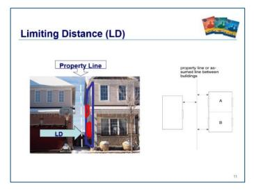
Limiting distance is defined in the NBC as the distance from an exposing building face to a property line, the centre line of a street, lane, or public thoroughfare, or to an imaginary line between 2 buildings or fire compartments on the same property, measured at right angles to the exposing building face. The NBC then places limits on the percentage of unprotected
