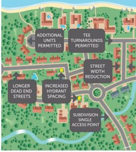
As a result of the life saving features of sprinklers, occupants have more time to safely selfevacuate. Sprinklers therefore are ideal alternatives when the following conditions exist: - inadequate water supplies for fire fighting - delayed response times for first responding units and/or effective firefighting force - inability to meet street width, grade, or lengths of cul de sacs - inability to meet the number of required egress routes - construction beginning prior to availability of
